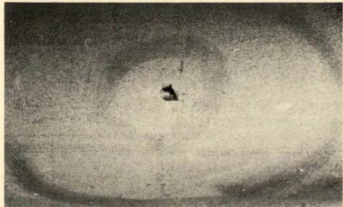
Top to bottom—High pressure fuel tube, dent in tube, cutaway showing hole and interior erosion of tube, exterior view of the hole.
